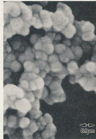
Figure 2. SEM photograph of the calcined 3 mol% yttria-stabilized zirconia powder
